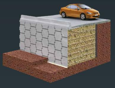
The original Reinforced Earth® technique combines select granular, engineered backfill with steel or synthetic tensile reinforcements and a modular facing system. This ideal combination creates a durable, mass gravity retaining wall.
