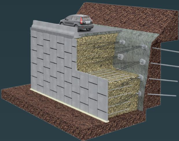
TerraLink® allows building new Reinforced Earth type walls connected to retaining structures such as slopes stabilized by nailing or existing retaining wall.
