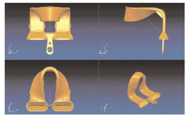
Developed by the Reinforced Earth research and development division, the Omega connexion is an anchoring system for synthetic reinforcements that is cast directly into the panel during the prefabrication stage.
