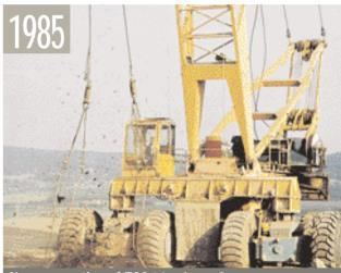
New generation of 700 t/m dynamic compaction cranes.
