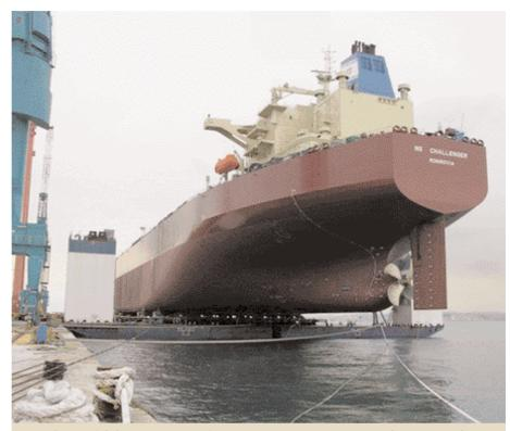
The Air Pad Sliding system (APS) developed by Hebetec uses jacks and air pads to launch boats that are built on dry docks.
